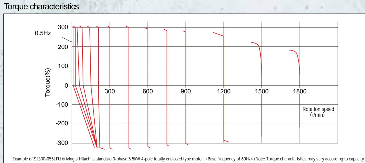
*Speed regulation at low speed has been drastically improved to enhance process stability and precision.*
