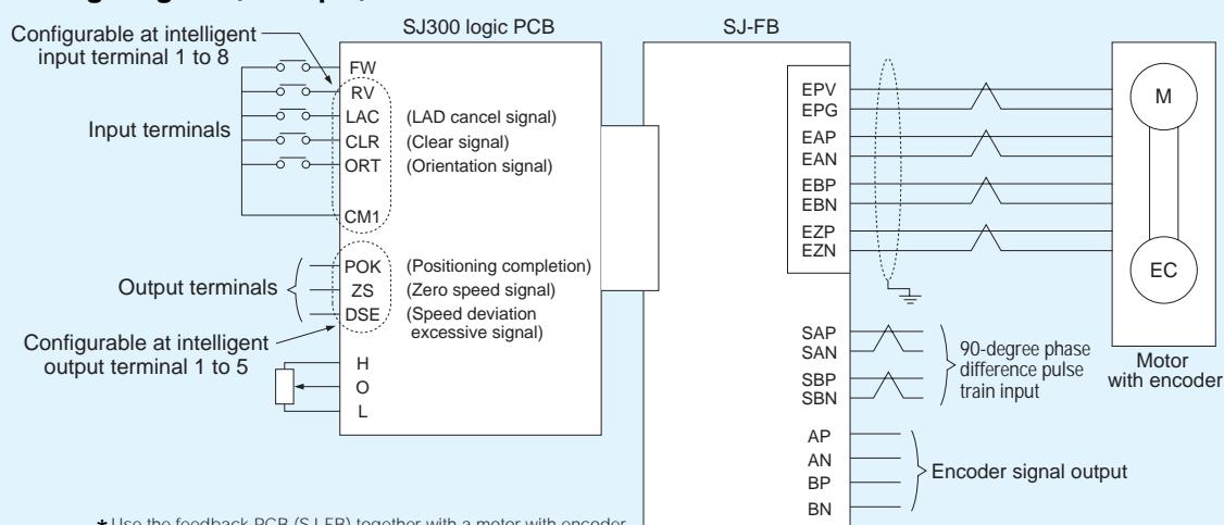
\* Use the feedback PCB (SJ-FB) together with a motor with encoder.
