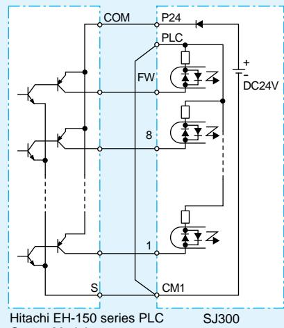
(Note: Place short-circuit bar between PLC and CM1 instead of P24 and PLC)
