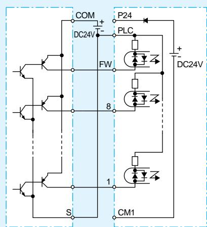
(Note: Remove short-circuit bar between P24 and PLC)
