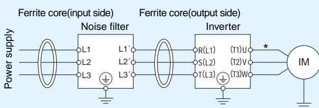
\*Use shielded wires between the inverter and the motor, and make sure not to exceed 20m(66ft).
